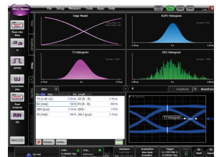
Figure 4: 32 Gb/s PRBS 211-1 showing 138 fs RJ(rms).
