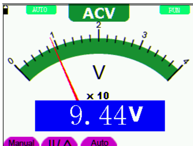
Figure 26: AC Voltage Measurement
