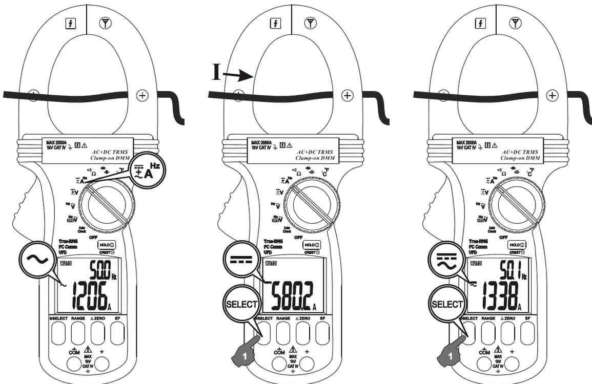
Input is made through the clamp jaws for non-invasive current measurements. Defaults at **ACA<sup>Hz</sup>** Function. Press **SELECT** button momentarily and release to select the subject functions in sequence.
