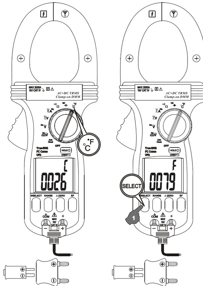
Defaults at **°C** (Celsius) readings. Press **SELECT** button momentarily and release to select **°F** (Fahrenheit) readings. Inputs are made through the test leads terminals. Be sure to insert the banana plug type-K temperature bead probe AMD 9023 with correct **+** **-** polarities. You can also use a plug adapter AMD 9024 (Optional purchase) with banana pins to type-K socket to adapt other type-K standard mini plug temperature probes.
