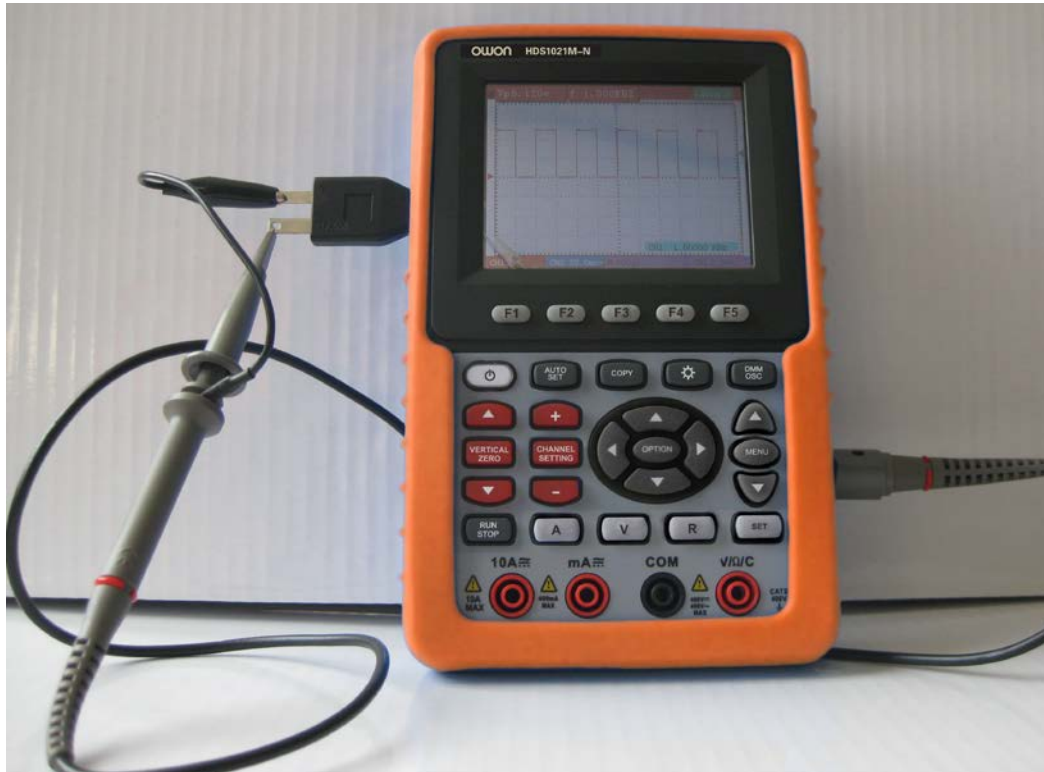
Fig.3. The connection of Square-wave test signal
