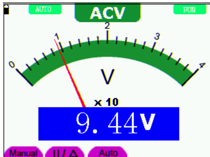
Figure 23: AC Voltage Measurement
