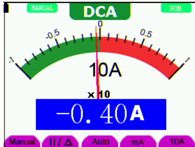
Figure 25: DC Current Measurement for 10A
