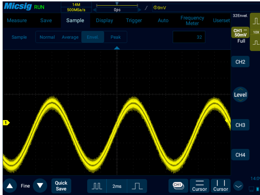
Figure 11-8 AM Signal in Envelope Sampling Mode (32)
