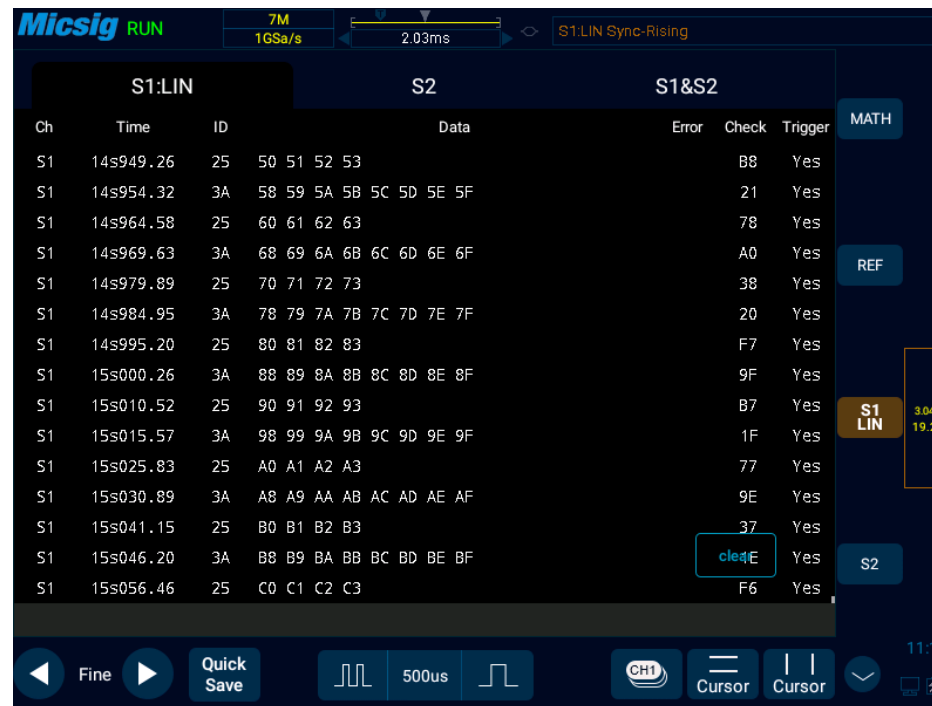
Figure 12-13 LIN Text Interface
