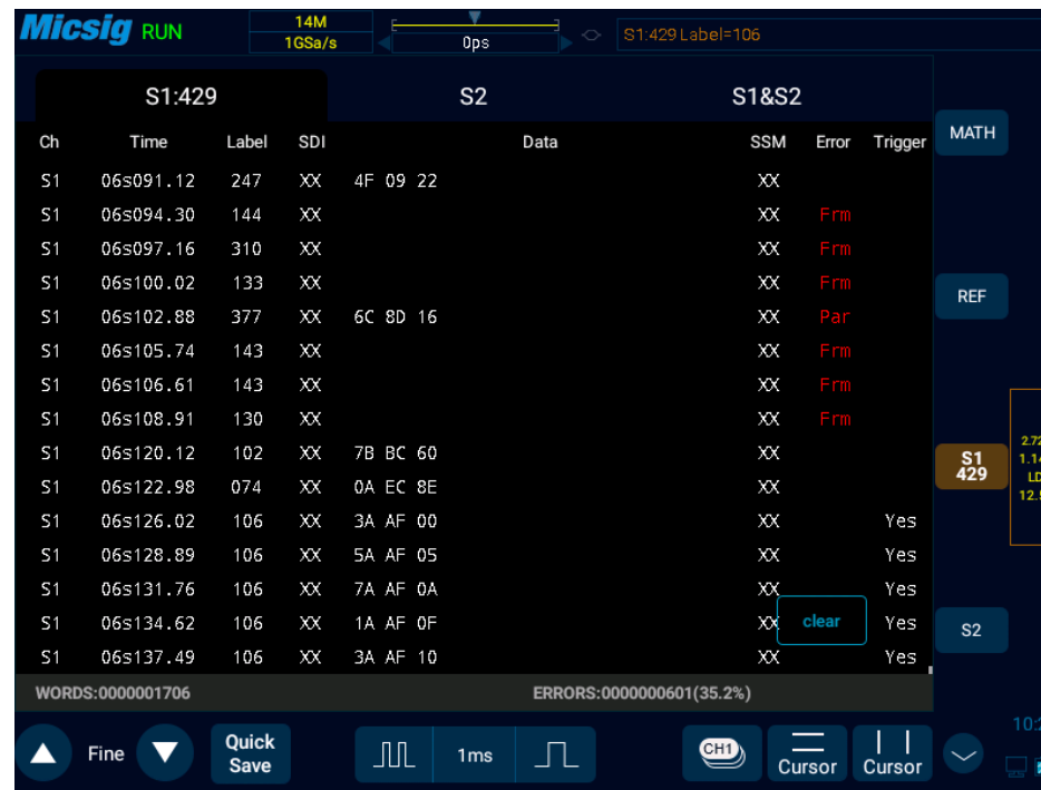
Figure 12-29 ARINC429 Text Interface
