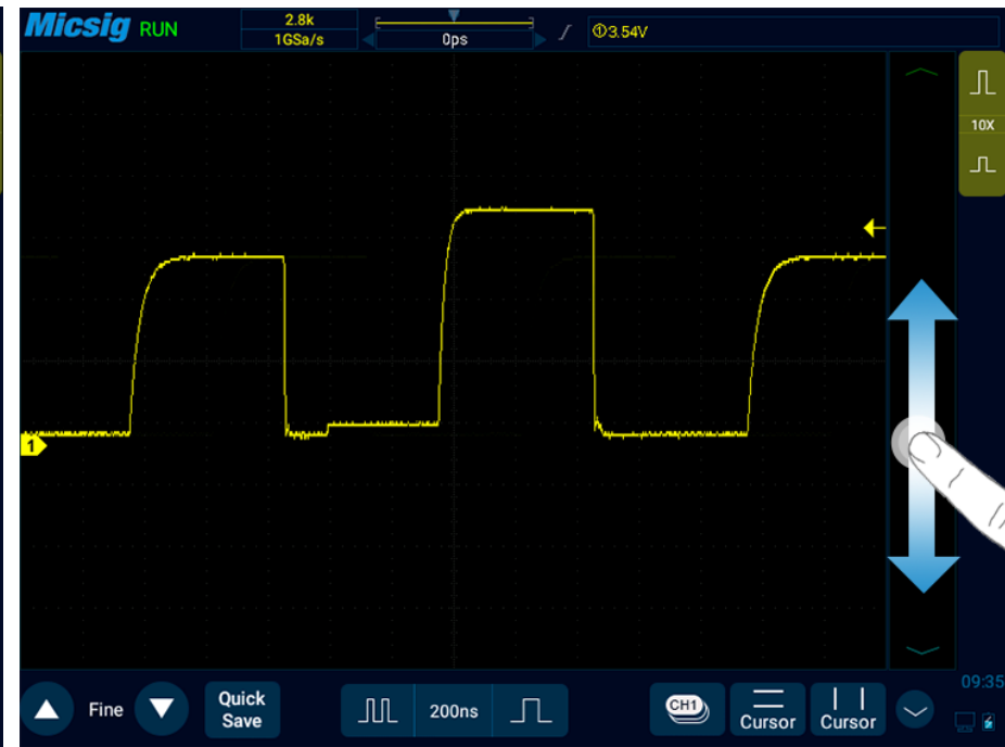
Figure 6-4 Abnormal Signal Captured by Setting Trigger Level
