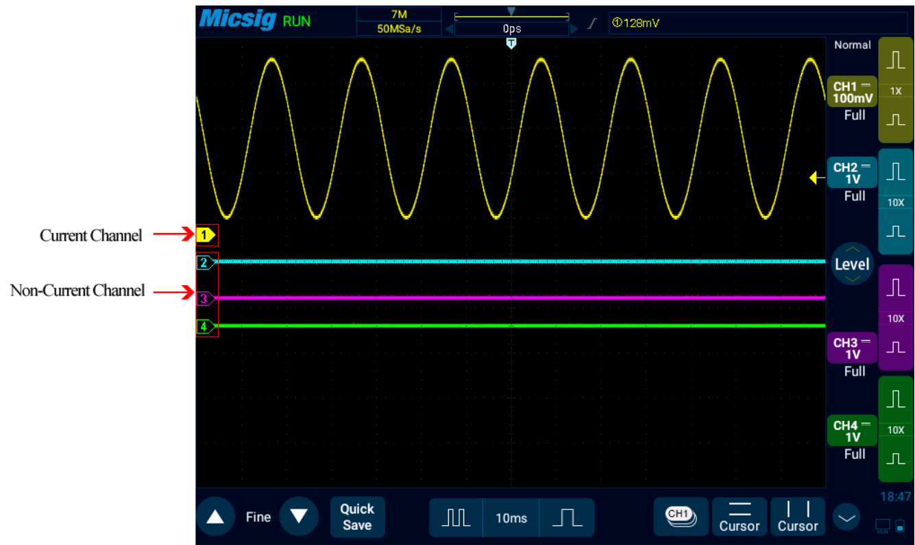
Figure 5-2 Current Channel and Non-Current Channel
