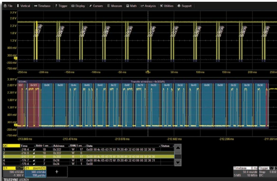
View decoded protocol information on top of physical layer waveforms and trigger on protocol specific messages.
